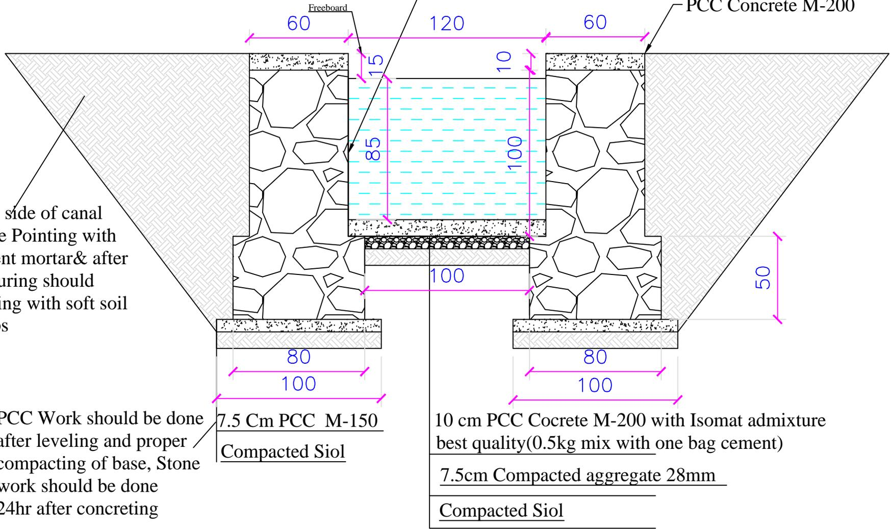
Both out side of canal should be Pointing with 1:3 cement mortar & after proper curing should back filling with soft soil in 3 Steps
