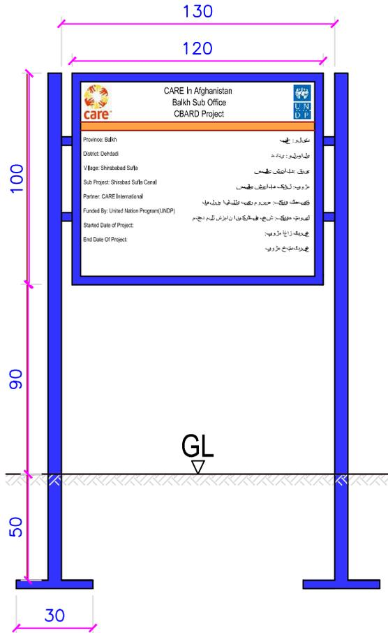
Profile (40x40x2)mm 5cm Length Should be proper weld with poles and sign board fram
