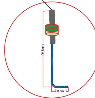
Column Fixing Side Iron Sheet
