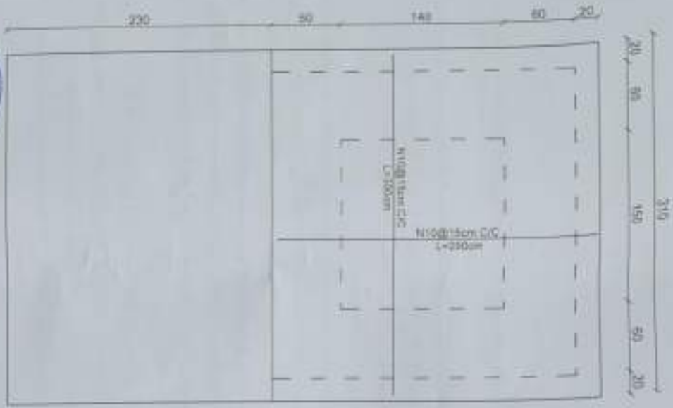
Second Floor Slab Reel Plan
